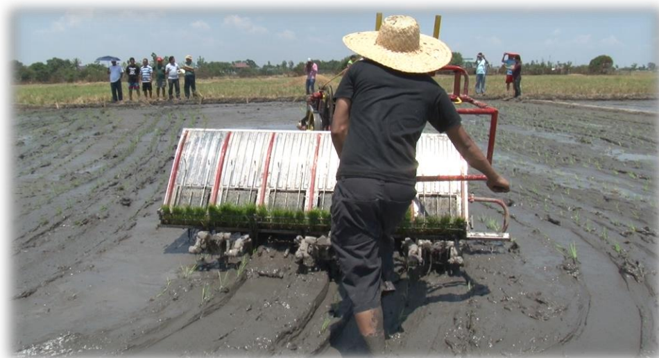
Figure 4. Field testing of the hand tractor-attached transplanter prototype in Amucao, Tarlac.
